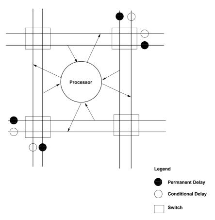
Fig. 3.12. PR-MESH Architecture (1 Node)
