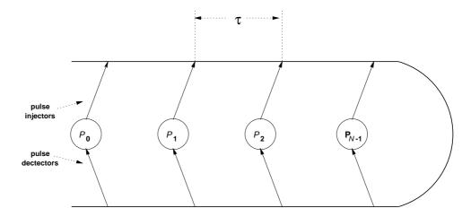
Fig. 2.2. Folded (Single) Bus Configuration
