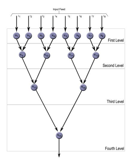
FIG. 4.1. Illustration of the parallel summation algorithm.
