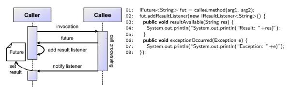
Fig. 4.1: Asynchronous method invocation with future return value
