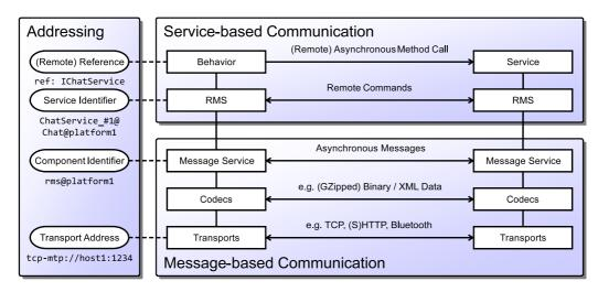
Fig. 5.2: Jadex communication stack
