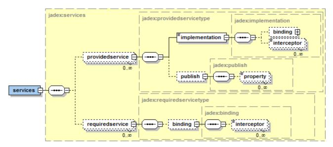
Fig. 4.4: Provided and required service specification
