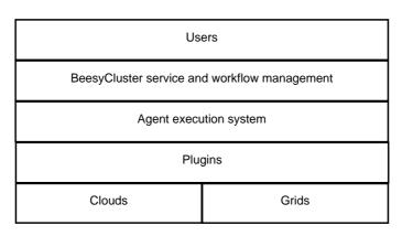
Fig. 4.4: Layers of the proposed architecture for running workflow applications on clouds and grids at the same time
