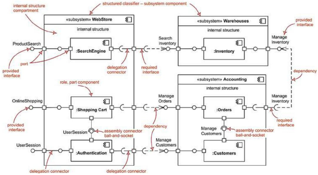
Fig. 2.2: Structure diagram of the element component.
