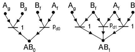
FIG. 5.5. P-graph model of a single comparator test
