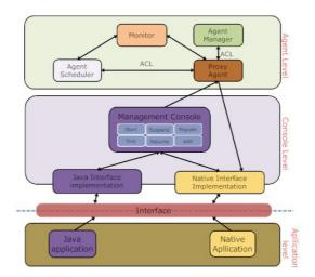
FIG. 4.1. Software Architecture
