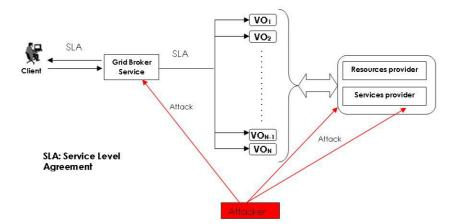
FIG. 4.1. Basic components of a grid system
