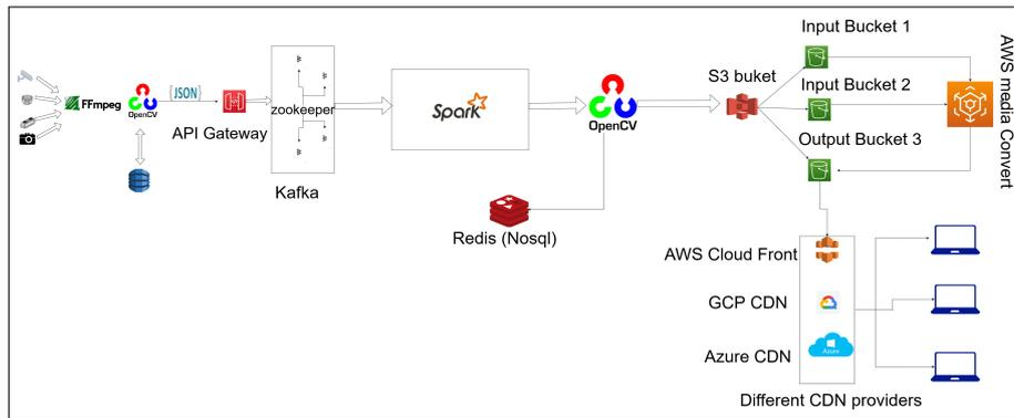
FIG. 5.3. System Architecture
