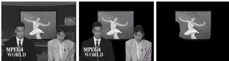
FIG. 5.3. Adaptation on system level: object based adaptation (from [12])
