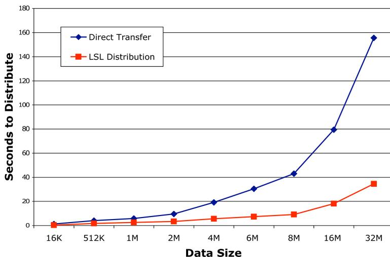
FIG. 5.1. *Distribution Times for 18 Hosts*
