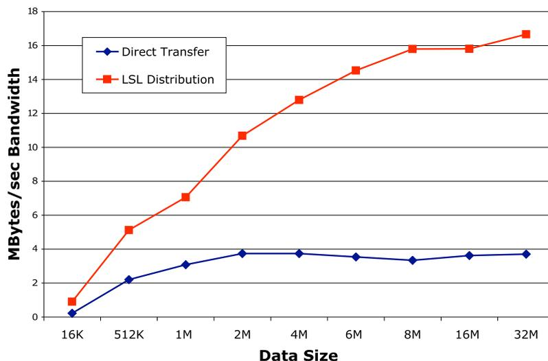
FIG. 5.3. *Delivered Bandwidth of Distribution Tree (18 Hosts)*
