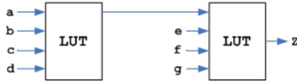
FIG. 2.1. Seven input bits to occupy two LUTs
