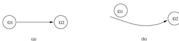
FIG. 4.4. (a) Connected dataflow graphs and (b) Non-connected Lazy graphs. In scenario (a), G_2 needs to wait for G_1 . This scenario is applicable if the Operand port in G_2 is strict. In scenario (b), G_2 can start before G_1 executes. The Operand port in G_2 is non-strict in this scenario. In the first case, G_1 is the Predecessor graph and G_2 is the Successor graph. In the second case (b), G_1 becomes Successor and G_2 becomes Predecessor.
