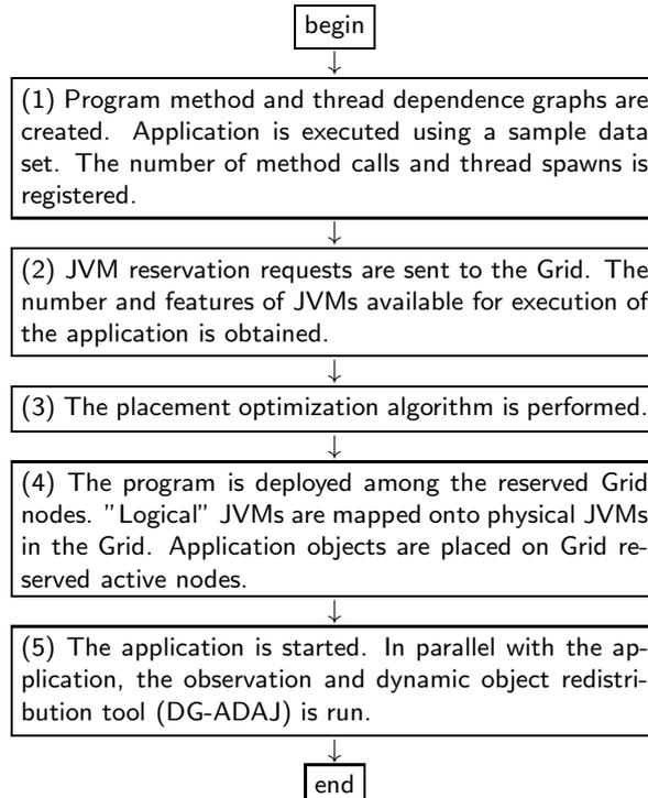
FIG. 3.1. *The control flow of an application execution.*
