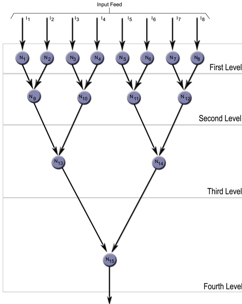
FIG. 4.1. Illustration of the parallel summation algorithm.
