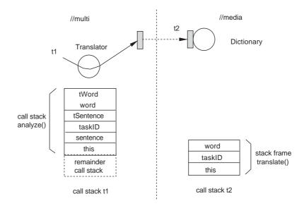
FIG. 5.4. Distributed Execution—state before Capturing.
