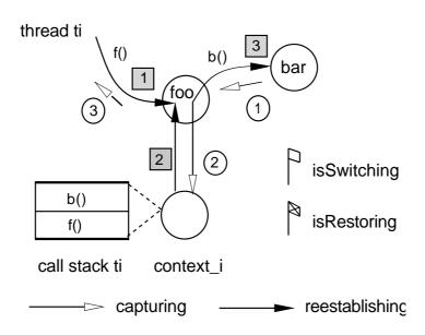
FIG. 2.1. Thread Capturing/Reestablishing in Brakes.
