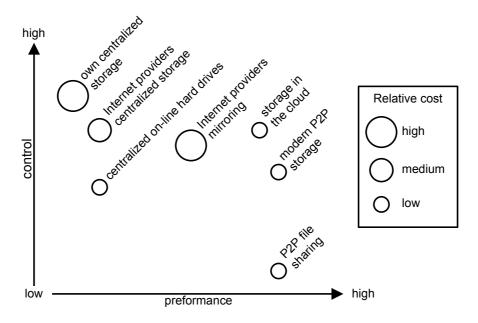
FIG. 2.1. Control/performance tradeoff in storage solutions
