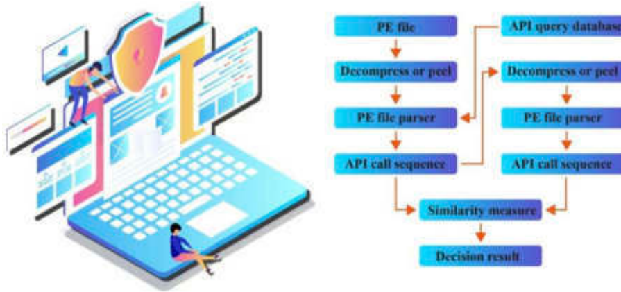
Fig. 3.1: Main structure of DMAV system
